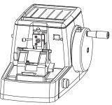
Clean the instrument regularly as part of your normal housekeeping routine, paying particular attention to the removal of wax from the area around the Knife Holder. Always remove the knife or blade, apply the handwheel brake, and lock the Knife Holder on its dovetail slide before starting any maintenance.
