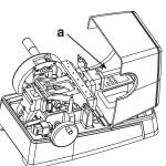
Find the tilt adjuster screws 1 and 2 in the bag of accessories and screw them into position on the Orientation Head. The shorter screw (screw 1) fits in the top hole and adjusts the vertical tilt angle of the Orientation Head; the longer screw (screw 2) fits in the hole in the left hand side of the Orientation Head and adjusts the horizontal angle.
