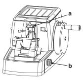
To make the maximum specimen travel available before starting a session of sectioning, turn the Coarse Advance Knob (*c*) to move the specimen head backwards. When only red shows on the indicator on top of the specimen arm (*a*), the end of travel is near in the rewind direction. The alarm sounds when the limit is reached.
