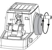
The specimen is retracted from the knife edge during the return stroke to prevent the specimen brushing against the back of the knife blade.
