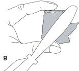
Use a scraper, plastic spatula or ParaTrimmer to remove excess wax from the sides, ends, and back of the cassette (g). The cassette must be able to mount squarely on the Specimen Clamp.
