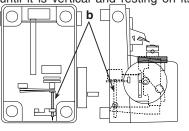
Loosen the two Knife Clamp Screws at the front of the Solid Knife Holder by turning them anti-clockwise *(b)*.
