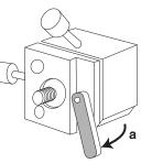
Fit the Specimen Clamp on the threaded bolt at the end of the Orientation Head, then screw it clockwise to tighten it in position *(b)*.
