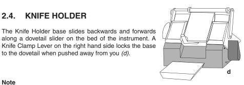
along a dovetail slider on the bed of the instrument. A Knife Clamp Lever on the right hand side locks the base to the dovetail when pushed away from you (d).
