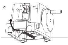
Remove the Top Tray from the instrument (e). Access to the transit fixings is via the outer cover of the instrument. This cover is retained by two spring clips that connect with shaped pillars mounted on the main frame inside.
