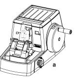
Release the handwheel brake and turn the handwheel clockwise until the handle of the handwheel is in the 2 o'clock position, and the specimen is just about to be cut.
